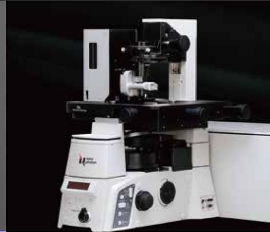
Tip-enhanced Raman Scattering Microscope
